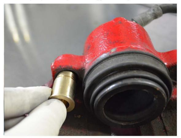
The bushings should go in by hand. If they need to be pushed in with more force than your fingers, Please clean the bore of any debris using a file or sandpaper. If they still do not slide in,
