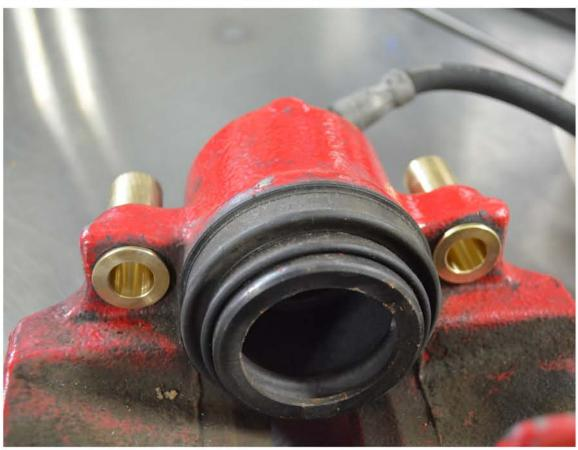
Using a snap ring plier, install the the snap rings along the ridge on the bushing.
