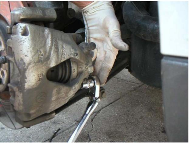
Remove the pins completely by pulling them out of the stock rubber bushings. You will not be reusing the stock pins.
