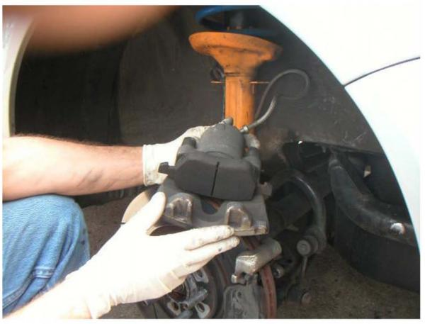
Remove the inner brake pad from the piston by prying outward.
