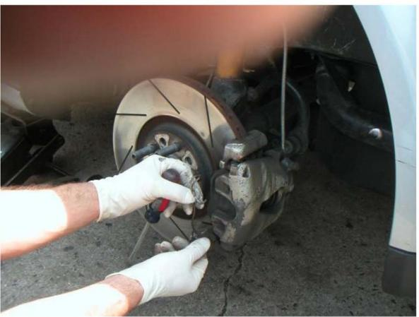
Next, locate the stock caliper guide pins on the rear of the caliper. You might have to remove the plastic caps which cover the pins.
