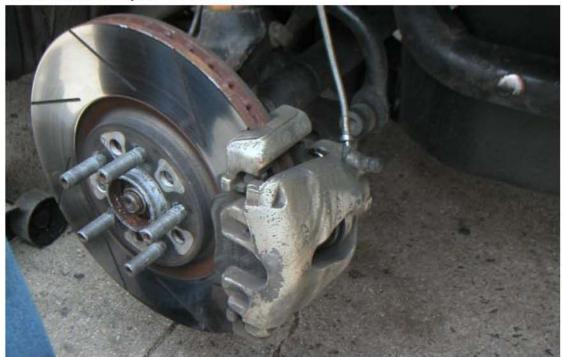
Coat the guide pins with anti-seize or the provided grease.
