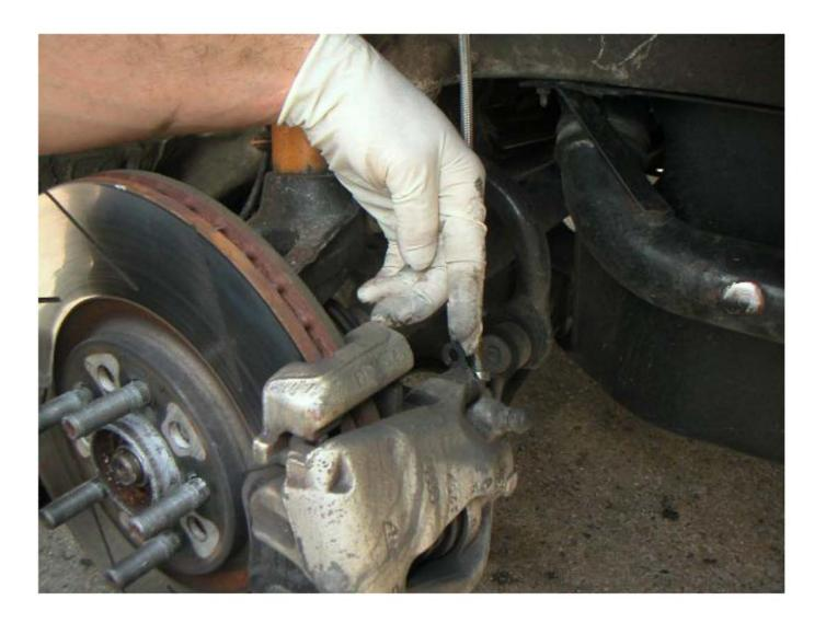
Remove the caps, and loosen the pins with a 7mm hex drive socket.
