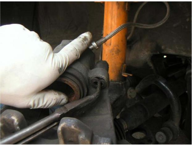
Insert the Tyrolsport bushing with the larger side facing the inside of caliper.
