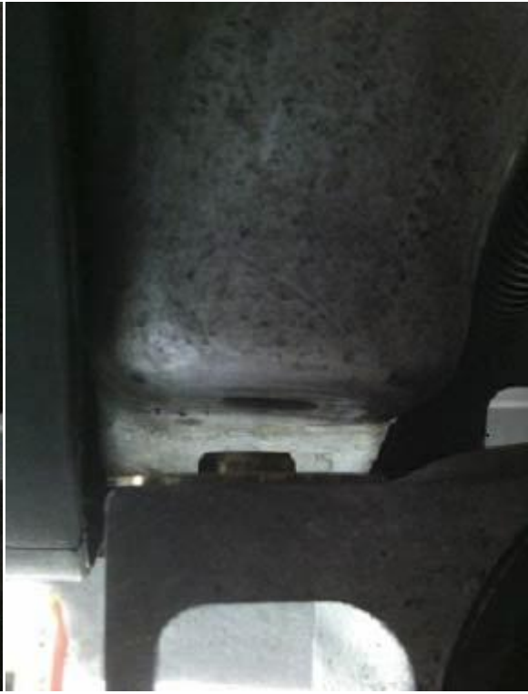
Top collar installed in control arm bushing housing.
