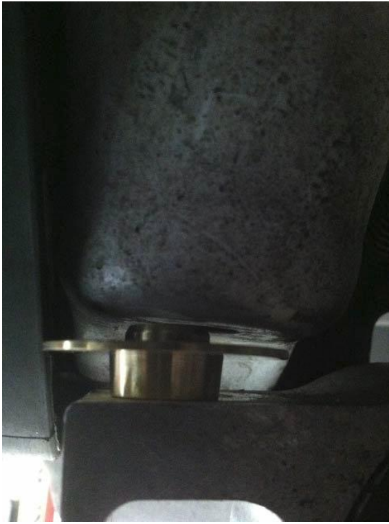
Direction of top collar between control arm bushing and body.
