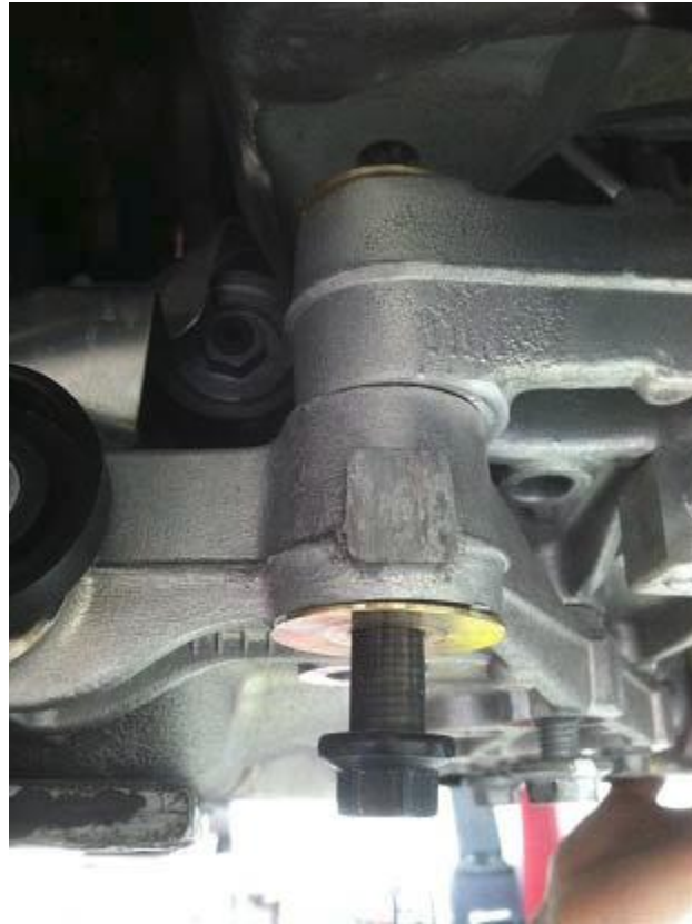
Both collars installed with bolt.
